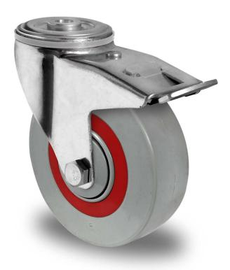
**Product SKU** BPH35WC100M6N2R32 Standard **DIN EN 12532** Compliance Series M6N2 Fastening Bolt fastening Brake and back brake Direction Material of the polyamide (PA) wheel center Wheel Tread polyamide (PA) tread Temperature -20°C to +80°C range Wheel Diameter 100mm Load Capacity 160kg **Total Hight** 127mm Width of Tread 36mm wheel hub Width 40mm Offset 40mm **Fastening Bolt** 13mm **Hole Diameter** Swivel Radius 127mm Wheel Bolt Size M8 **Bushing** 12mm Diameter Wheel Bearing roller bearing
